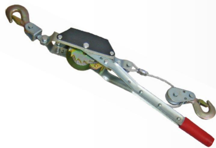
The image shows a hand-operated winch with a red handle, a silver metal body, and a hook. It has a pulley system and a gear mechanism.
